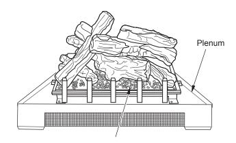
Figure 43 - Placing Ember Material on Burner
